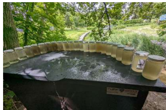
Water Samples – Turbidity is shown to increase left to right during a storm event.
